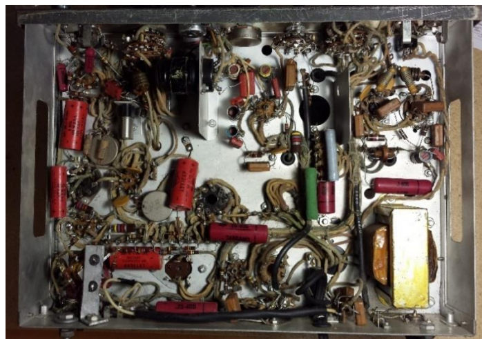
Under chassis before re-capping. Fairly clean except for dusty wiring. Note custom antenna relay bracket at lower left.
